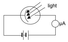
Light of different frequencies are incident on the aluminium cathode of a photo-cell and the kinetic energy of the ejected photo-electrons are determined. The graph below is drawn according to the data collected from the investigation.
