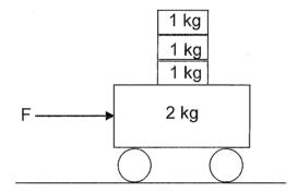
A force of magnitude F is applied to the 2 kg trolley. The trolley experiences an acceleration of *a*. If one of the 1 kg mass pieces falls off while F is still applied to the 2 kg trolley, the 2 kg trolley will accelerate at . . .
