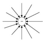
✓ Correct shape. Lines must not cross and must touch sphere
