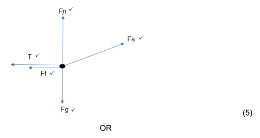
ACCEPT the labelled free-body diagram where the applied force is resolved into horizontal and vertical components ( $F_{ax}$  and  $F_{ay}$ )
