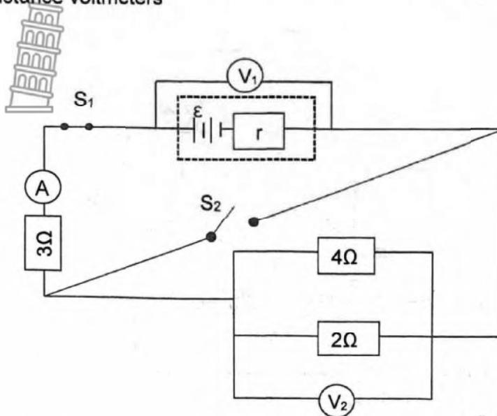
When switch  $S_1$  is **closed** and switch  $S_2$  is **open**, the ammeter reads 2,48 A.
