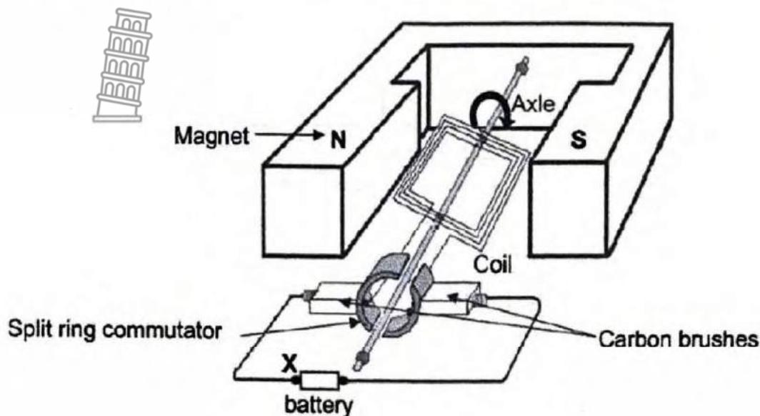
9.1.1 The coil rotates in a clockwise direction as indicated in the diagram above. What is the polarity of the pole of the battery labelled X? Choose from POSITIVE or NEGATIVE (2)
