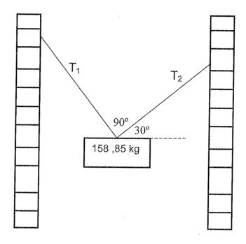
The angle between the cables,  $T_1$  and  $T_2$  is 90°. The angle between cable  $T_2$  and the horizontal is 30°. The net force acting on the object is zero.
