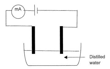
The  $Ba(OH)_2(aq)$  is added drop by drop to the distilled water and the ammeter reading is recorded after the addition of each drop.
