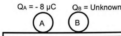
The spheres are brought into contact and thereafter separated. Each sphere now has  $1,25 \times 10^{13}$  excess electrons.
